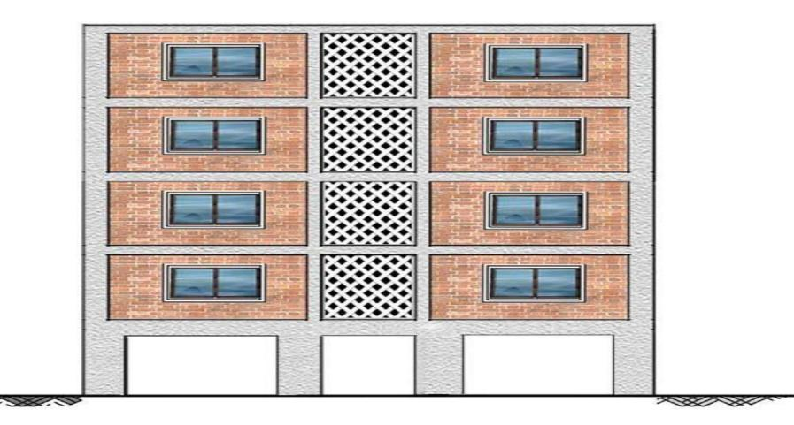
The size of the ground storey beams and columns is increased to have the stiffness of the ground storey comparable with upper storeys
