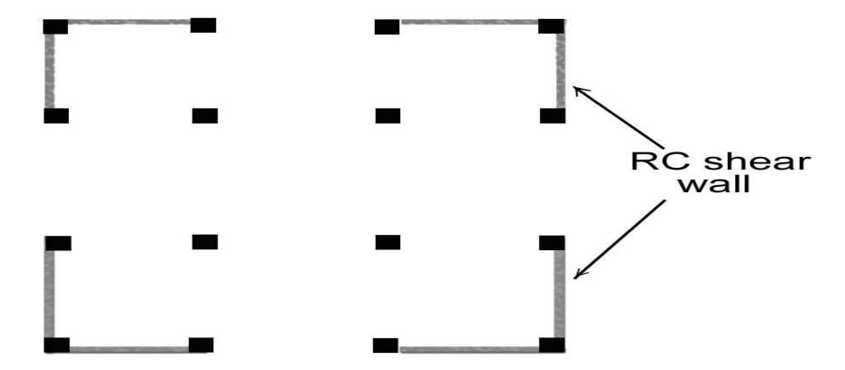
The ground storey should be provided with shear walls to increase the stiffness at ground storey
