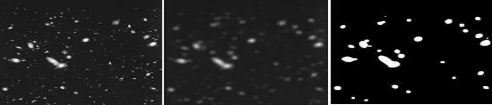
Image from Hubble telescope, image processed by 5x5 averaging window, and image after thresholding (nasa)
