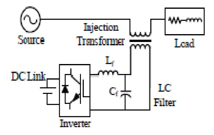
The Dynamic Voltage Restorer (DVR), also referred to as the Series Voltage Booster (SVB) or the Static Series Compensator (SSC), is a device that utilizes solid state (or static) power electronic components, and is connected in series to the utility primary distribution circuit. The DVR provides three phase controllable voltage, whose vector (magnitude and angle) adds to the source voltage to restore the load voltage to pre-sag conditions.
