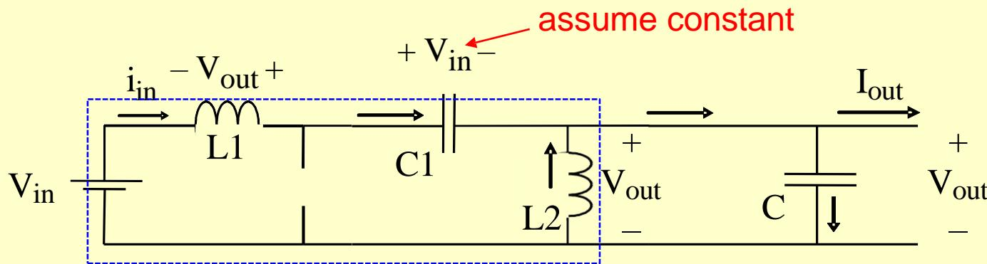
$C_1$  and  $C$  are charging.  $L_1$  and  $L_2$  are discharging.
