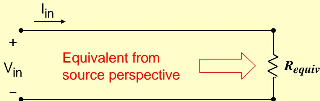
$$R_{equiv} = \frac{V_{in}}{I_{in}} = \frac{\frac{(1-D)V_{out}}{D}}{\frac{DI_{out}}{(1-D)}} = \left(\frac{1-D}{D}\right)^2 \bullet \frac{V_{out}}{I_{out}} = \left(\frac{1-D}{D}\right)^2 R_{load}$$
