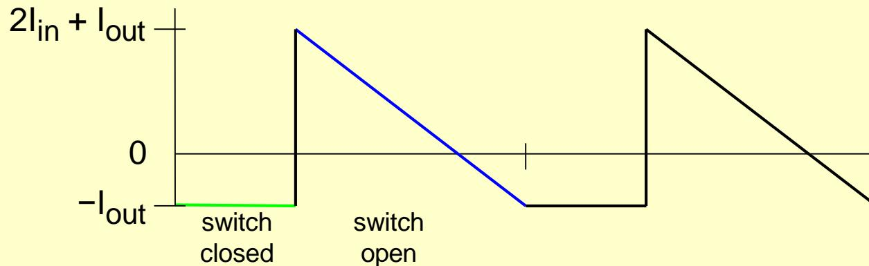
$$I_{in} = \frac{DI_{out}}{1-D}, I_{out} = \frac{(1-D)I_{in}}{D}$$
