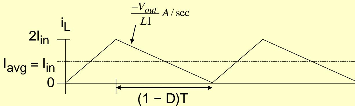
$$2I_{in} = \frac{V_{out}}{L1_{boundary}} \bullet (1 - D)T = \frac{\frac{DV_{in}}{1 - D}}{L1_{boundary}} \bullet (1 - D)T = \frac{V_{in}D}{L1_{boundary}f}$$
