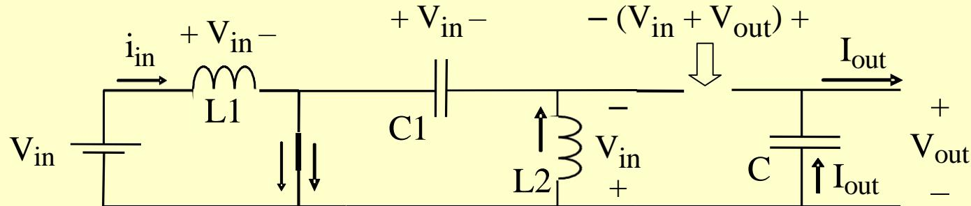
$i_{L1}$  and  $i_{L2}$  are ramping up (charging).  $C1$  is charging  $L2$
