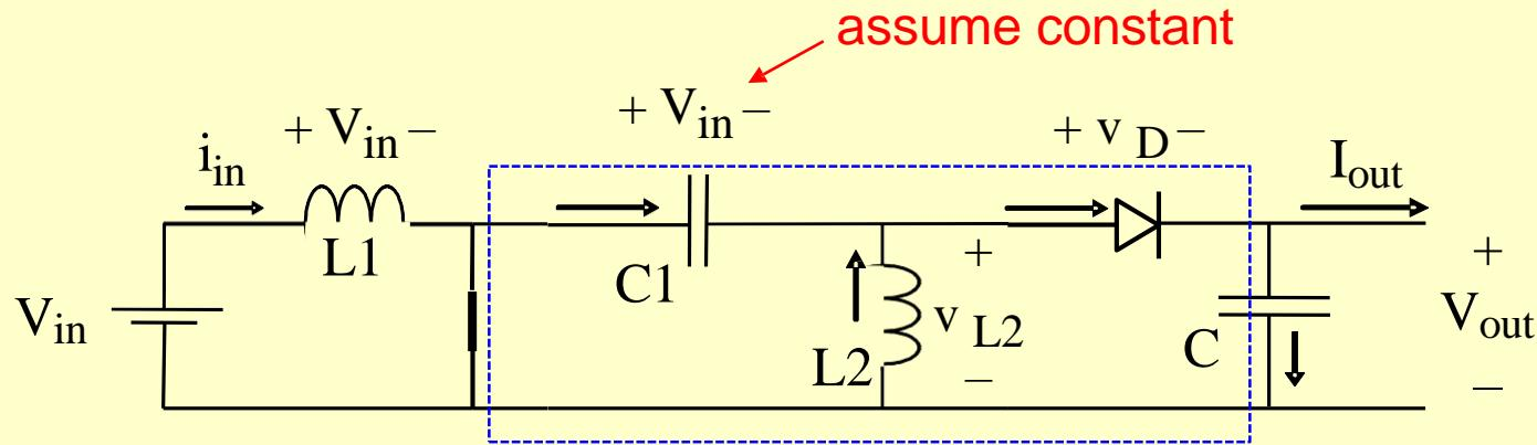
KVL shows that  $v_D = -(V_{in} + V_{out})$ ,
