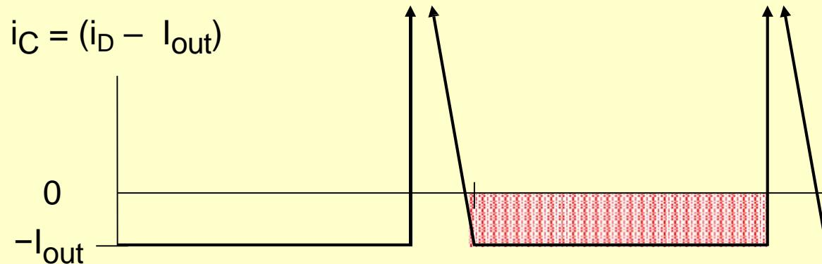
The worst case is where  $D \rightarrow 1$ , where output capacitor C provides  $I_{out}$  for most of the period. Then,
