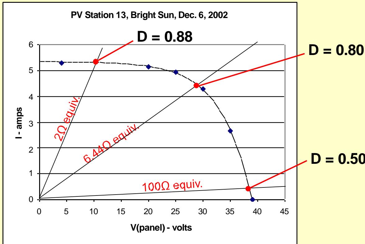
With a  $100\Omega$  load resistor attached, raising  $D$  from 0 to 1 moves the solar panel load from the open circuit condition to the short circuit condition
