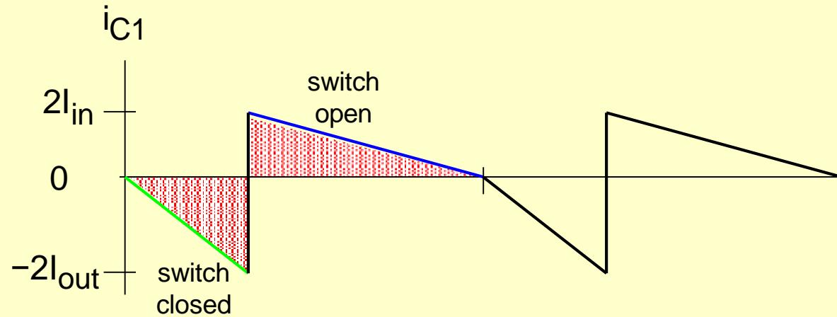
$$\Delta V = \frac{\Delta Q}{C1} = \frac{I_{out} \bullet DT}{C1} = \frac{I_{in} \bullet (1-D)T}{C1}$$
