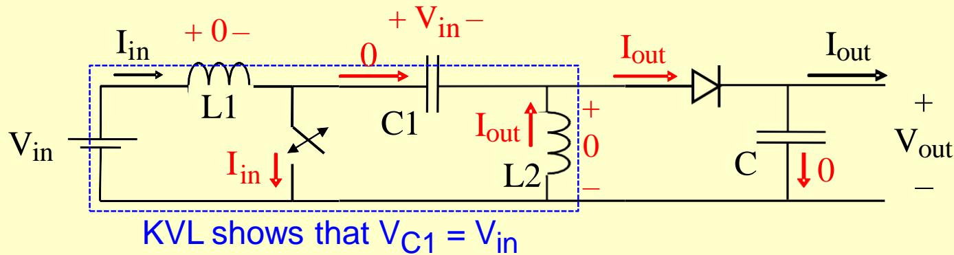
Interestingly, no average current passes from the source side, through  $C_1$ , to the load side, and yet this is a “DC - DC” converter
