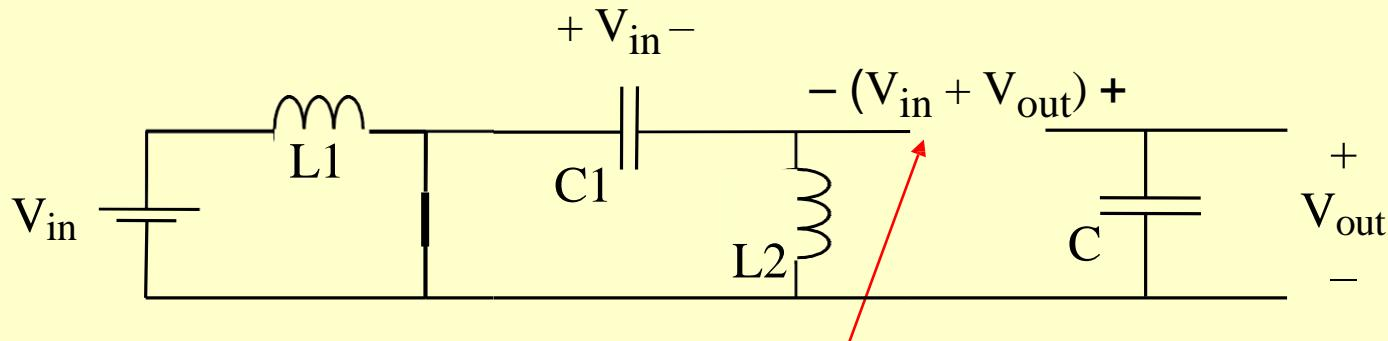
MOSFET and diode see  $(V_{in} + V_{out})$
