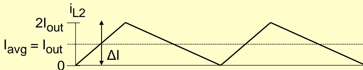
$$I_{L2rms}^2 = I_{out}^2 + \frac{1}{12}(2\Delta I_{out})^2 = \frac{4}{3}I_{out}^2$$
