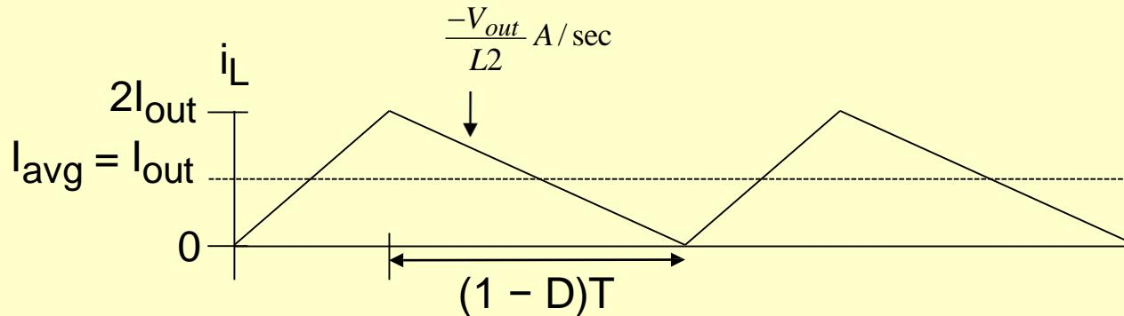
$$2I_{out} = \frac{V_{out}}{L2_{boundary}} \bullet (1 - D)T = \frac{V_{out}(1 - D)}{L2_{boundary} f}$$
